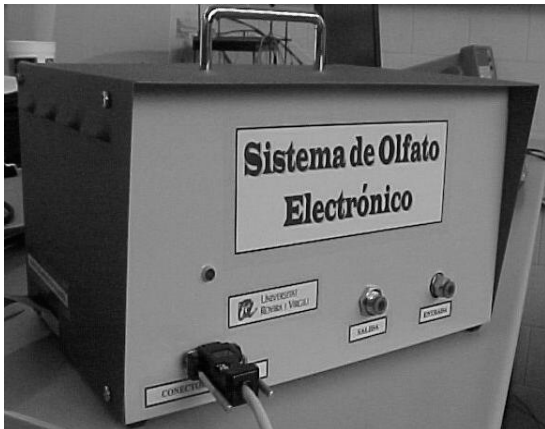
Fig.8. Photograph of the electronic nose system
